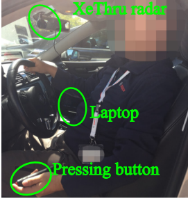
Figure 4: Equipment setup for the experiments
