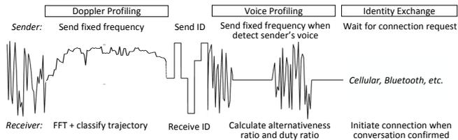
Fig. 11. Overall workflow of DopEnc and interactions between the sender and the receiver. The signals are depicted in frequency domain as detected by the receiver.
