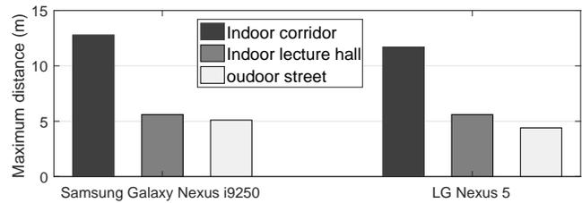
Fig. 15. Maximum transmission distance vs. different receivers and locations. We use another LG Nexus 5 as the transmitter
