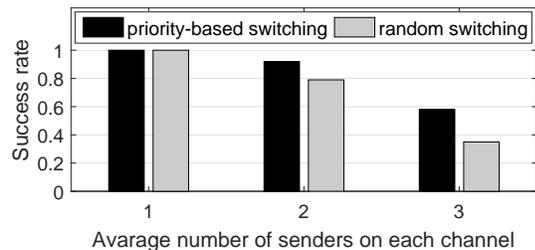
Fig. 19. Success rate of channel access vs. average number of senders per channel.
