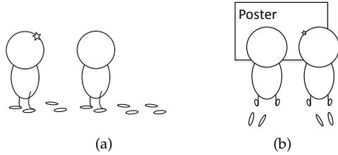
Fig. 9. Doppler profiling misidentifies “interactions” when (a) one person walks after the other, and (b) two persons walk towards a same target.
