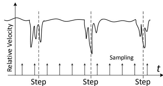
Fig. 6. Limited sampling rate contributes to occasional valleys. If the instantaneous body adjustment when human strikes the ground is sampled, then valley occurs.
