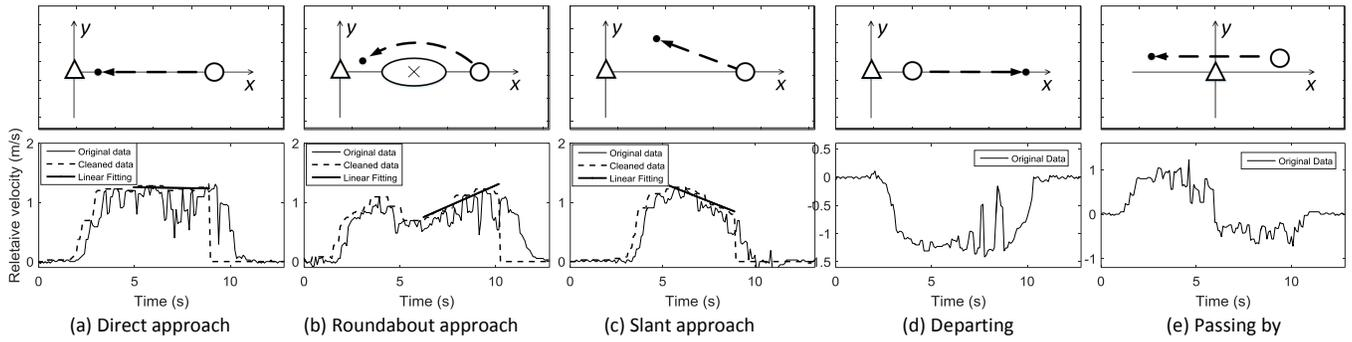
Fig. 8. Measured Doppler profiles of different categories of trajectories as well as the cleaned data.
